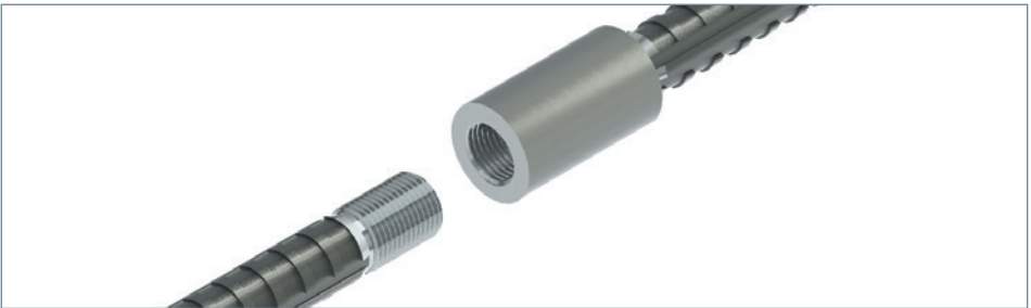
Figure 7. Parallel Thread System Parallel threads are applied directly to the rebar ends with the associated rebar coupler unit. The threads are typically rolled rather than cut onto the rebar.
