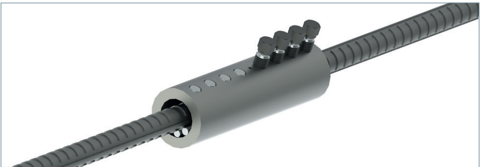
Figure 9. Bolted Sleeve System Requiring no rebar end preparation, this type of system can be used to connect rebar on site by placing the rebar within the sleeve and tightening the hexagonal headed screws until a specific torque is achieved, or the screw head shears off.
