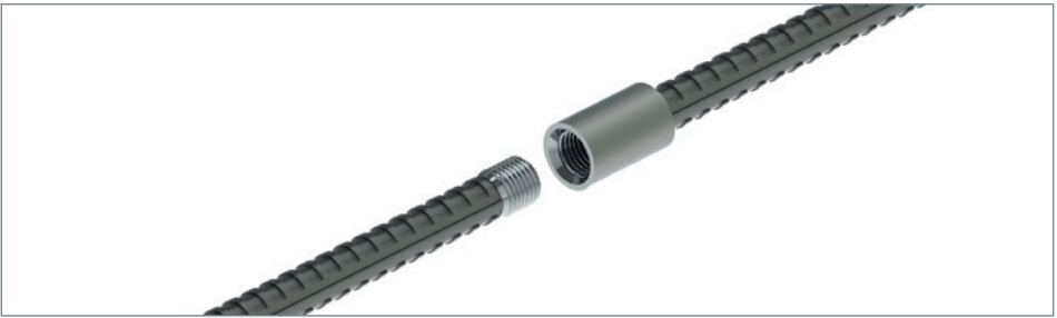
Figure 6. Parallel Threaded System on Upset Rebar Ends The ends of the rebar are cold forged to increase their diameter prior to threading
